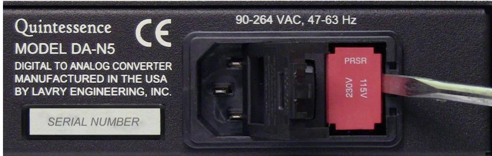
Always replace the fuses with the same value and type that was installed (Fast blow or Time Delay), or check the product information on our website for up-to-date information on fuse values. [lavryengineering.com](http://lavryengineering.com)
