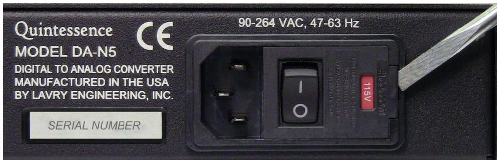
Once the latch releases, you can open the door completely by hand. This photo shows the door half-way open. The door latch is visible where it overlaps the red fuse holder:
