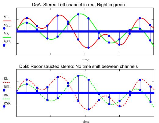
Given that stereo audio tracks are sampled simultaneously and reconstructed simultaneously, there is no relative time shift between channels. Clearly, the time between samples for a 44.1 KHz system is 22.7µsec. For 384 KHz the time is 2.6µsec. But it does not matter. Decreasing the time between samples does nothing to alter the accuracy of the timing relationship between channels!
