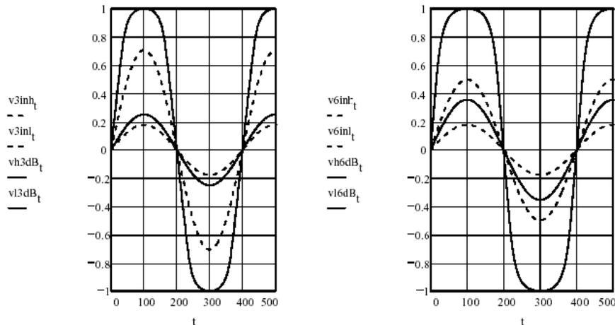
The soft saturation algorithm provides a "soft limiter" function (aimed at making "hotter recording"). The function provides several advantages over conventional analog limiters.
